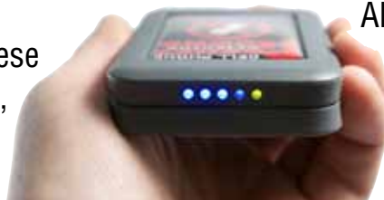
PocketHound™ detects RF signature of any cell phone up to 75 feet away
