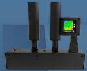
Integrated thermographic antenna identifies heat sources generated by lighted warning devices.
