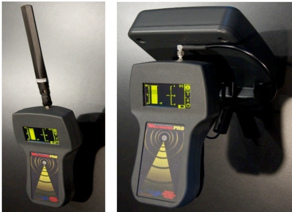
Figure 1. Wolfhound-PRO Unit may be used with the Omnidirectional or Direction Finding (DF) Antenna
