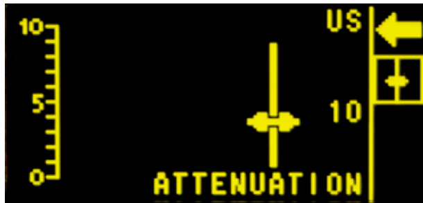
Figure 20. ATTENUATION screen (set to ~ 10dB)
