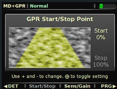
Individual GPR setting of the start and stop points
